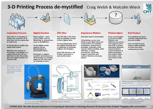
Schematic of 3-D printing process
