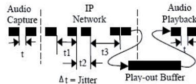
**Figure 1: Relationship between play-out buffer usage and Jitter Inter-arrival time**
