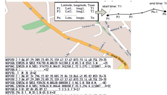
Fig 2: GPS data and path of a moving object
