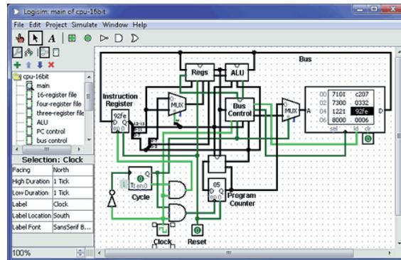
There are some excellent tools for learners of digital electronics, Logisim for example. Logisim is a very accessible software application that demonstrates the dynamic behavior of digital circuits.
