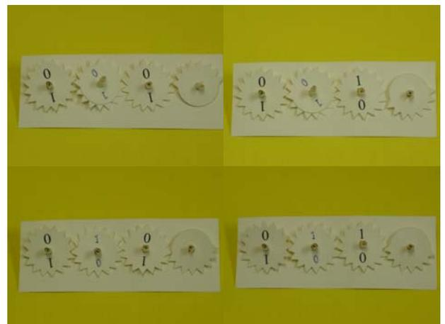
**Figure 5: Binary Gears, showing successive disengagement each half-turn; the third binary digit's half-gear is obscured by its lower-valued neighbour's transmission gear, which is co-axial**
