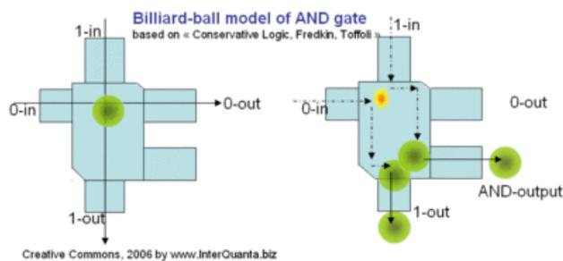
**Figure 1: Billiard Ball Computer implementation of an AND gate**
