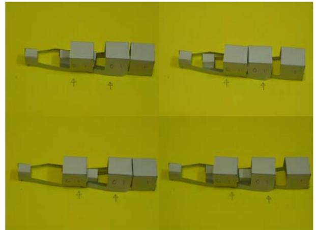
**Figure 4: Push-Pull Binary Blocks – a very early prototype showing the required binary counting sequence, but with no clutch mechanism yet in place**
