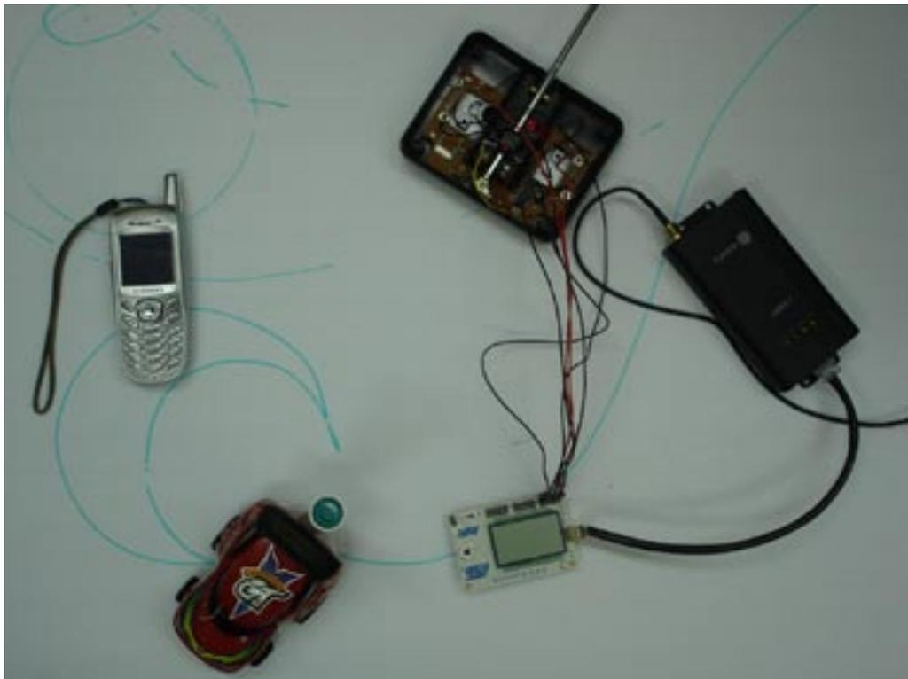
**Figure 2: Components for Project 1 (clockwise from top left: cellphone, adapted remote control, cell receiver, ATMELEK butterfly, remote control car).**
