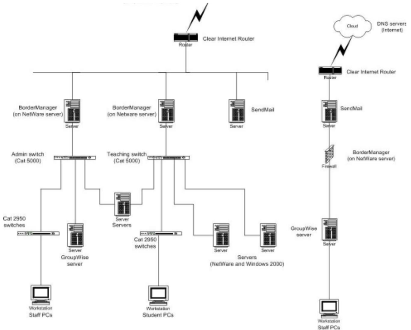
**Figure2. A simplified view of the Wintec network a) Physical and b) Logical. Knowledge of the network assists with the ICF design by identifying points of access, infection and control.**
