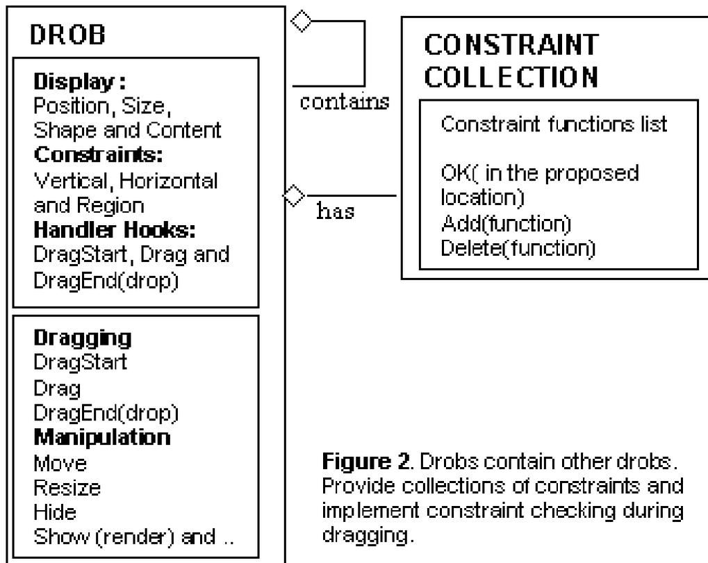
**Figure 2.** Drobs contain other drobs. Provide collections of constraints and implement constraint checking during dragging.
