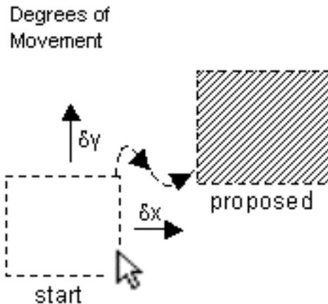
**Figure 1.** Dragging from a start position to a proposed destination. Constraints are expressed in vertical and horizontal terms as well as regions. A constraint may prevent the proposed destination.
