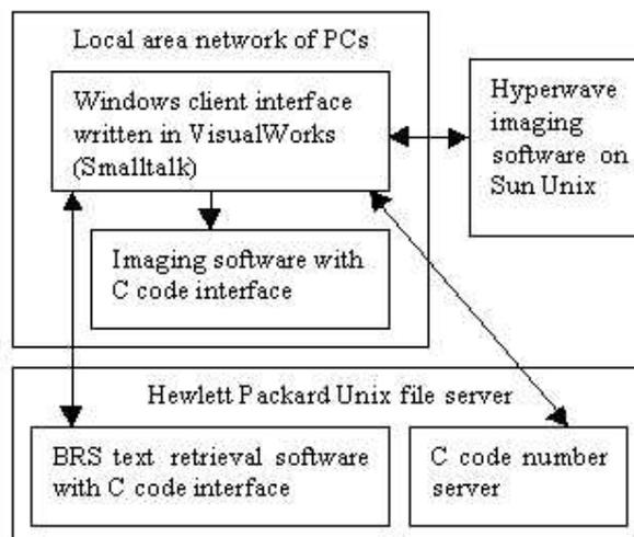
Figure 1. Te Kahui System Architecture.
